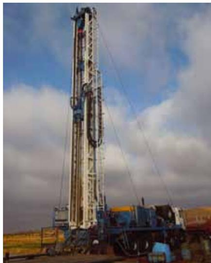
and foam pump. A deck mounted Deutz engine powers the rig and optimizes fuel consumption and maintenance cost. The G-50 mounted on a heavy duty 8 x 8 four axles Astra Truck is highly mobile and can reach difficult-to-access sites. ■
